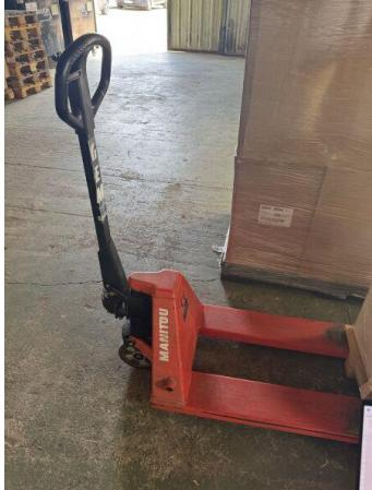
A red manual pallet truck (transpalette) with 'MANITOU' branding on the forks. It is shown in a warehouse setting, positioned next to a stack of wooden crates.                     |
