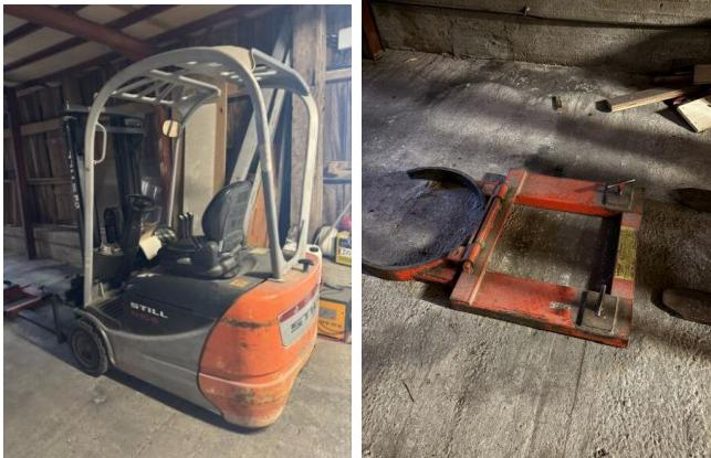
Two images showing an orange forklift (chariot élévateur) with a white protective cage and its attachment, a red cylindrical drum holder (broche porte fût), lying on the ground. |
